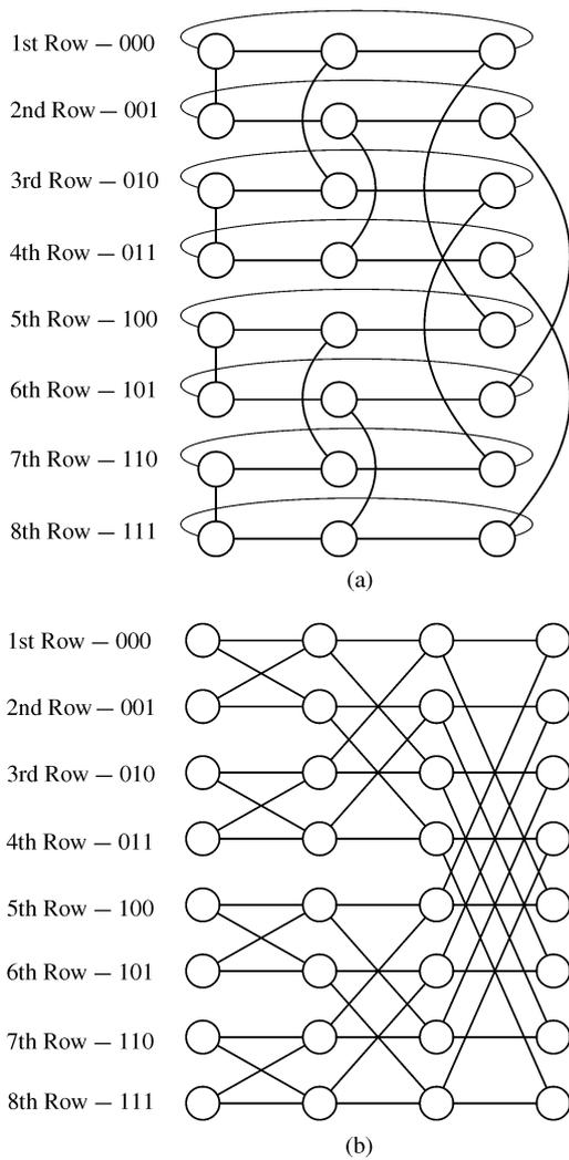
Fig.2. (a) Two-dimensional layout of a 3-dimensional CCC network. (b) Classical representation of an 8-input Butterfly network.
