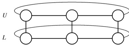
Fig.3. Reduced graph of a 3-dimensional CCC network.
