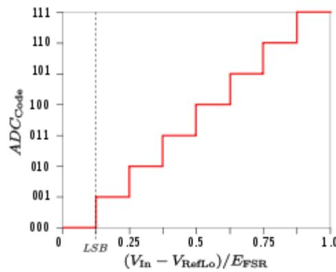
**Quantization error:** rounding error between the analog input voltage to the ADC and the output digitized value.
