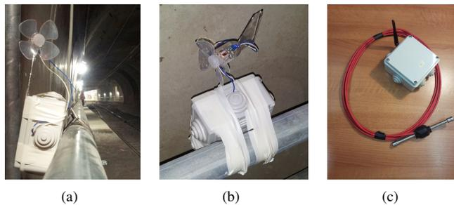
Fig. 1. (a)(b) Snapshots of nodes deployed in an underground train tunnel in Rome; (c) A sensor node interfaced with a vibrating wire strain gauge.
