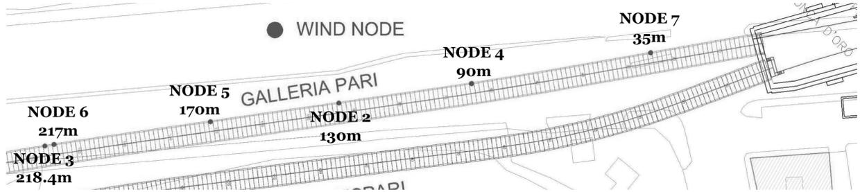
Fig. 2. Motes deployed in the tunnel and their distances from the train station. (Site plan courtesy of Roma Metropolitana and Tre Esse Engineering).
